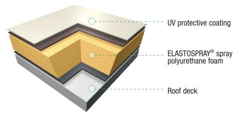
The ELASTOSPRAY<sup>®</sup> spray-applied polyurethane foam (SPF) roofing system from BASF Polyurethane Foam Enterprises LLC boasts high eco-efficiency and return on investment according to an Eco-Efficiency Analysis. ELASTOSPRAY roofs include seamless polyurethane foam insulation with a fluid-applied ELASTOCOAT<sup>™</sup> elastomeric membrane.
